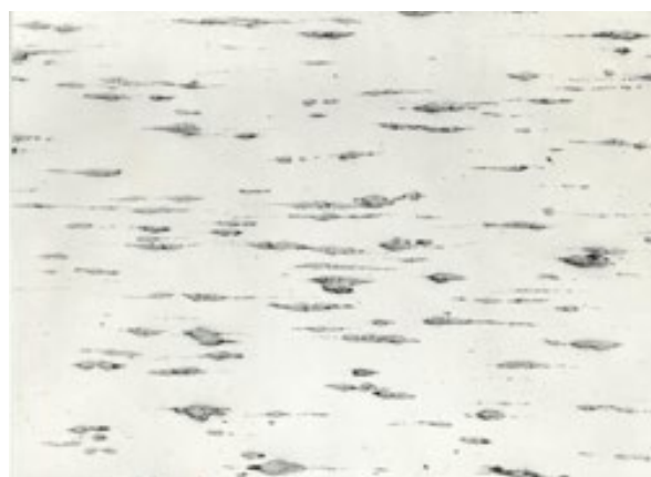
Figure 2. Microstructure of Ingot R-2, rolled to ¼-inch strip at 1850F (1010C).
